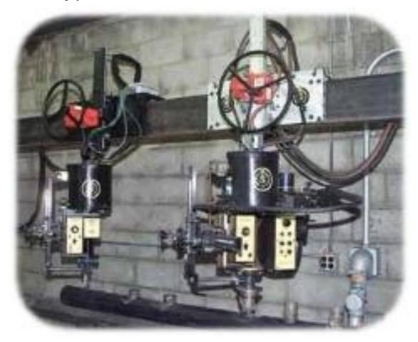
Made by Cypress Welding Equipment, Inc., the CB-1P plasma hole cutter with the CW-5 Series Circle Welder, when equipped with the optional CWO-4530 Carriage which is mounted on a standard monorail, the plasma cutter & the circle welder can move anywhere along the length of pipe.
