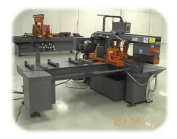
The HEM Horizontal Pivot Band Saw Model H90A-C Series is the latest version in computerized band saws. This saw features:
