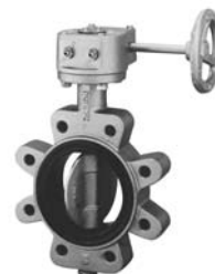
Code # 6123-E-G Body Style: Lug Design Disc: Aluminum Bronze Liner: EDPM Operator: Gear Operator
