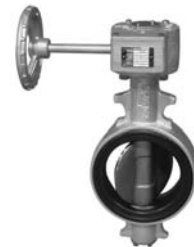
Code # 5123-E-G Body Style: Wafer Design Disc: Aluminum Bronze Liner: EDPM Operator: Gear Operator
