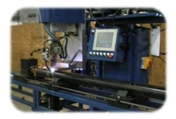
The "Univeral Welding System" developed by North Alabama Pipe Corporation, combines a plasma hole cutter with a MIG circle welder coupled with a roller table system with an automatic clamping device; all computer controlled. This machine is capable of handling 1-1/4" - 8" pipe.
