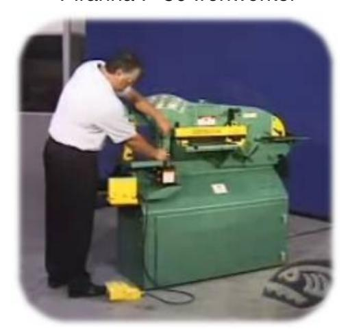
The Piranha Single Operator Ironworker Series has more standard workstations than any other ironworker in its class. Capabilities include punching, bending, bar shear, angle shear, round bar shear, and an integrated coper/notcher.
