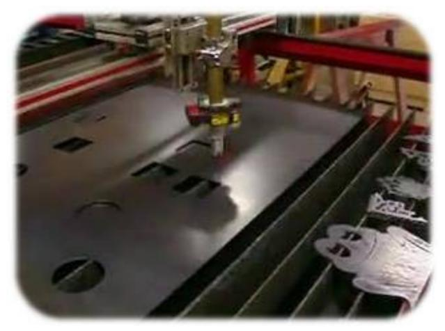
This CNC style Plasma Cutting table can handle steel plates up to 5' wide and 10' long with a maximum plate thickness of 1". It is capable of cutting mild steel, stainless steel and most alloys.
