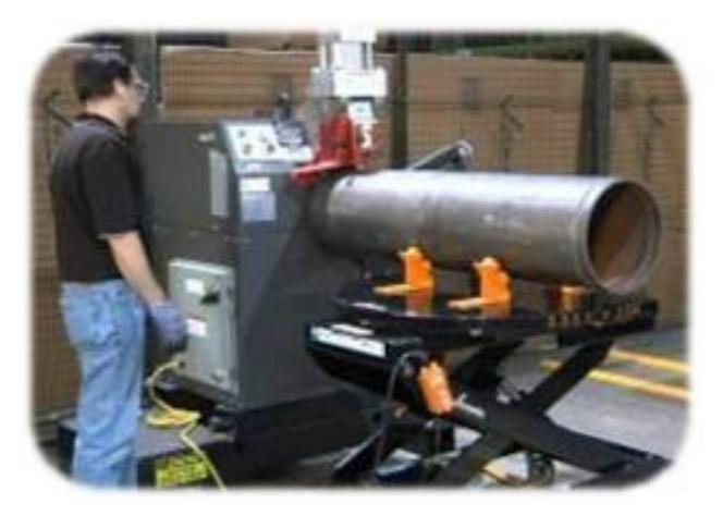
Production roll grooving equipment suitable for mechanical fabrication shop applications are usually manufactured by Pace Machinery or Victaulic Company. These machines will roll groove carbon steel & stainless steel pipe thru 24" diameter and copper tubing thru 8" diameter.
