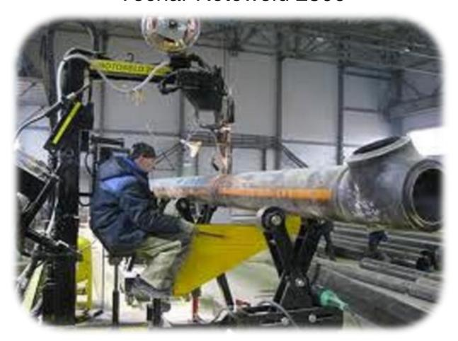
The Rotoweld 2500 is the latest version of the Rotoweld technology. It combines, into a single welding carriage, a complete SAW welding system for fill and cap passes together with Technar's vision-assisted STT automated root pass process.
