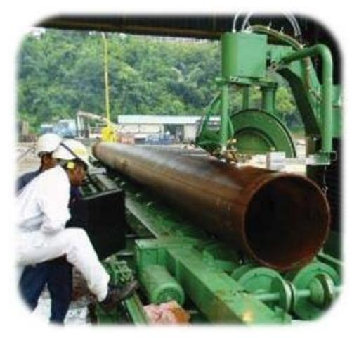
Vernon Tool now offers the MPM Series fully computerized pipe cutting machine. The 4 & 5 Axis versions feature servo driven rollers that fully support and rotate pipe during cutting and can be integrated with lifter conveyors for automatic loading & unloading.
